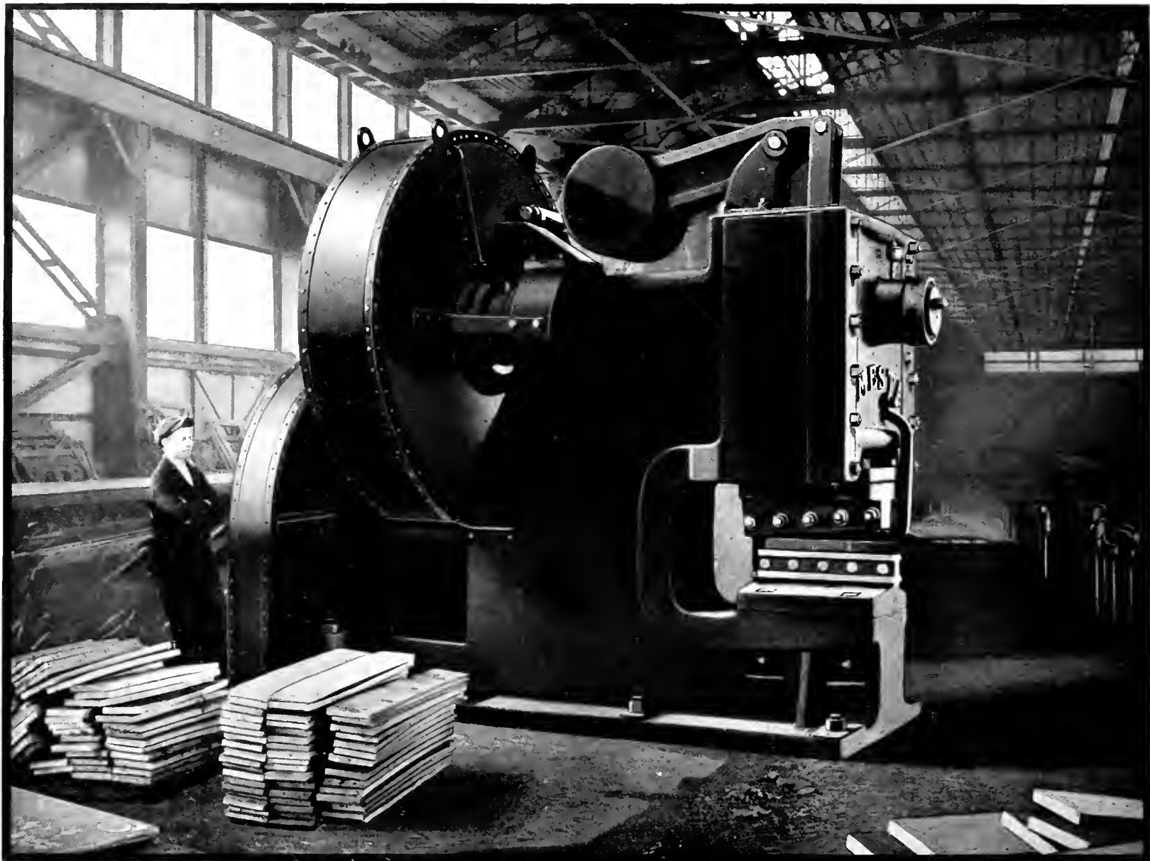
One of Five Mesta Vertical Open Throat Bar Shears Built for the Homestead Works of The Carnegie Steel Company
